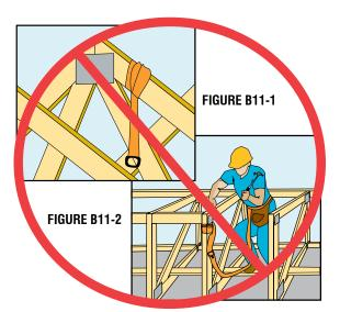
WARNING Roof and floor Trusses that are not properly braced per BCSI or sheathed are not able to resist lateral impact loads associated with falls. A falling worker attached to an inadequately braced set of Trusses could cause all the previously set Trusses to collapse in a domino effect.
