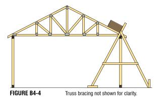
**DON'T** stack materials at or near the midspan of the Trusses. Never exceed stack heights per Table B4-1, unless alternative information is provided by the Building Designer, Truss Designer or Truss Manufacturer.
