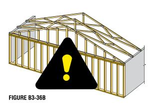
Special end wall Bracing design considerations are required by the Building Designer if the Gable End Frame profile does not match the adjacent Trusses.
