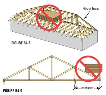
**DON'T** pile cut-off tile and/or other construction waste on Truss roofs.
