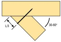
FIGURE B8-9 Corner jack to corner Girder Truss
