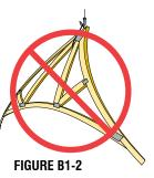
✓ Due to treatment effects, fire retardant treated Trusses require special care when handling to prevent chord and web member breakage. Limit exposure to the elements per manufacturer's recommendations.
