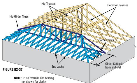
Install jacks while crane continues to hold Girder Truss in place.
