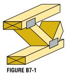
✓ The wider bearing surface (2.5" for 3x2 and 3.5" for 4x2), shallow depths (typically 24" or less) and relatively short spans (40° or less) make PCT
