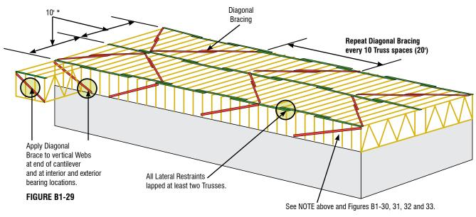
\*Top Chord Temporary Lateral Restraint spacing shall be 10' o.c. max.
