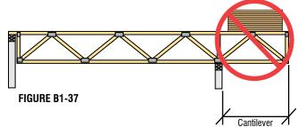
DON'T drop loads of any material on Trusses. Truss damage  $\odot$ from the impact is possible even if the weight of the material is small.
