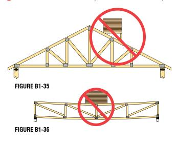
$\bigcirc$ **NEVER** stack materials on the cantilever or overhang of a Truss.
