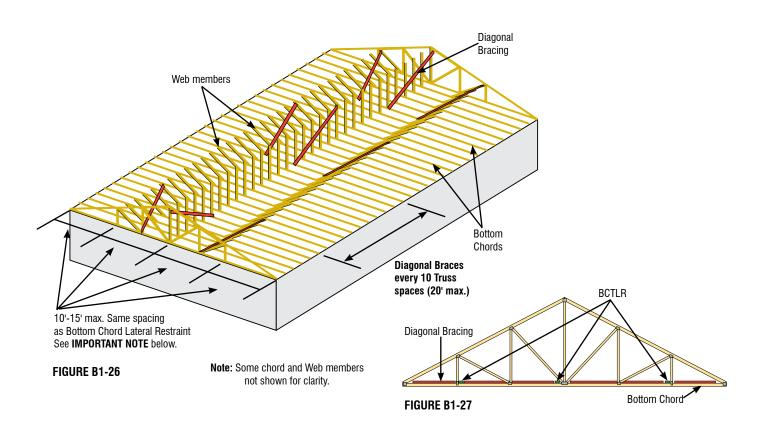
3) **BOTTOM CHORD TEMPORARY LATERAL RESTRAINT** (**BCTLR**) **AND DIAGONAL BRACING** is required to maintain oncenter spacing for the Bottom Chord and to laterally "stiffen" the group of Trusses. Place Continuous Lateral Restraint and Diagonal Bracing on top of the Bottom Chord (Figures B1-27 and 28). This material can be removed after the permanent ceiling Diaphragm is in place or remain to become part of the Permanent Building Stability Bracing (PBSB) system.
