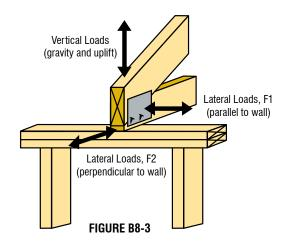
✓ Wind Loads acting on a Truss, as well as certain multi-span Truss applications supporting gravity Loads, can produce uplift reactions at Truss bearing locations. The magnitudes of these uplift reactions are typically provided on the Truss Design Drawing (TDD).
