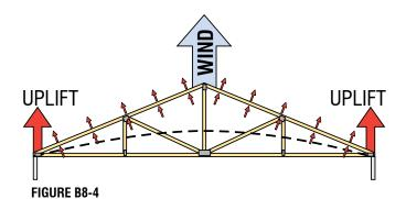
✓ Wind and seismic forces acting on the Building produce lateral Loads that are often transferred at the Truss bearing locations. The magnitude and direction of these wind and seismic Loads are to be provided by the Building Designer.
