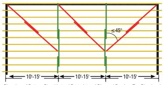
Plan view of Bottom Chord Lateral Restraint and Diagonal Bracing. Top Chord and Web Lateral Restraint and Diagonal Bracing not shown for clarity.
