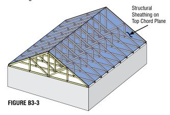
✓ Wood or metal Purlins are most often used in applications where Trusses are spaced greater than 24" o.c. The Purlins must be properly sized and fastened to the Top Chord of the Trusses in accordance with the specifications found in the Construction Documents. The Trusses must be designed so that the maximum allowable unbraced length for the Top Chord is greater than or equal to the on-center spacing of the Purlins.
