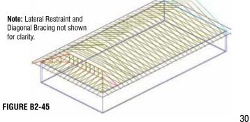
DON'T stack materials or stand at locations that will cause instability, such as on cantilevers, overhangs, end jacks or near truss-to-girder connections.
