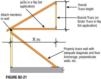
✓ X = wall setback (ft) = overall Truss height (ft-in) rounded to next full Truss Spacing (ft), or Girder Truss set back in hip end framing. For example, if the overall Truss height is 5'-6" and the Trusses are to be spaced at 2' on-center (o.c.), use a wall setback, X, of 6' (i.e., three Truss Spaces @ 2' = 6' > 5'-6").
