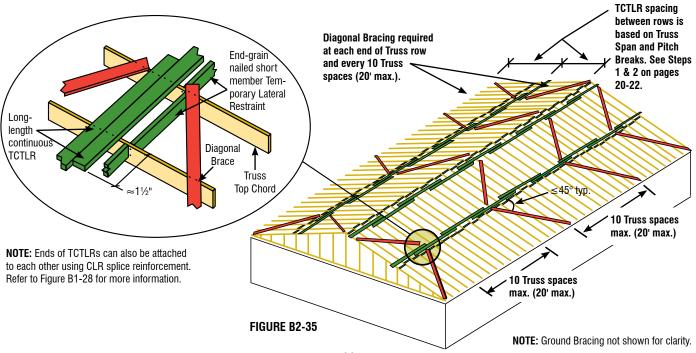
WARNING This Diagonal Bracing option can only be used if the Contractor installs long-length continuous TCTLR as indicated in Step B below.
