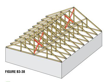
Sway bracing is typically installed on web members (verticals whenever possible) located at or near each row of Bottom Chord Lateral Restraint and should extend from the Top Chord Plane to the Bottom Chord Plane at right angles to the Trusses.
