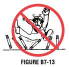
O DO NOT walk on unbraced Trusses.
