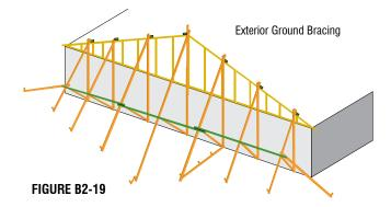
Example of first Truss installed with interior Ground Bracing to top of wall and back to floor below (see Figures B2-20 and 21).
