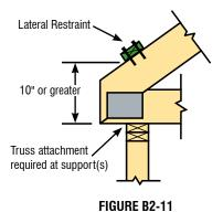
✓ For all bracing and Lateral Restraint members, nail as follows (except end-grain-nailed short member Lateral Restraints, which require 3 1/2" long deformed shank (i.e., ring- or screw-shank) nails):
