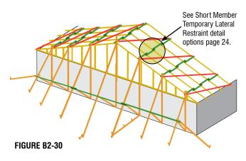
Example of Diagonal Bracing on first five Trusses with Ground Bracing to top of Building wall and back to floor below:
