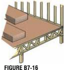
Position stacks of materials flat with the longest dimension perpendicular to the Trusses as shown in Figure B7-16.
