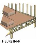
DON'T drop Loads of any materials on Trusses. Truss damage from the impact is possible even if the weight of the material is small.
