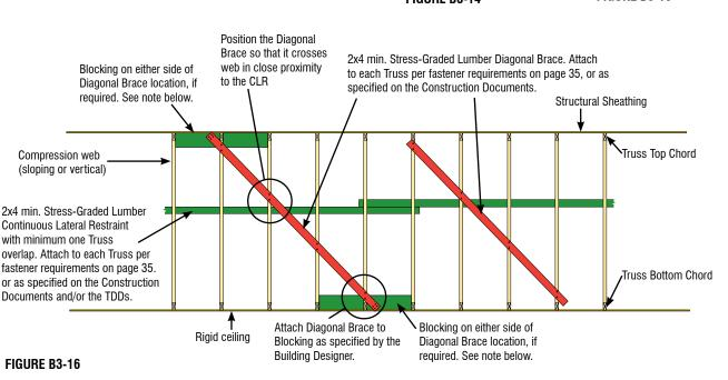
**Note:** To help transfer large Bracing forces into the roof and ceiling Diaphragms, dimension lumber Blocking may need to be installed between the Trusses on either side of the Diagonal Brace location as shown in Figure B3-16. Cut the Blocking to fit snuggly between the Trusses and attach to the Trusses and the Diaphragm. The Blocking helps to transfer the lateral Load directly from the Diagonal Brace into the Diaphragm.
