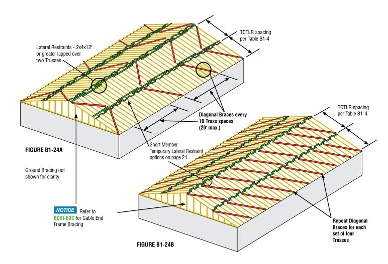
▲ WARNING Exact spacing between Trusses should be maintained as the Lateral Restraint and Diagonal Bracing is installed to avoid the hazardous practice of trying to remove this material to adjust spacing. This act of "adjusting spacing" can cause Trusses to topple if the restraint and Bracing is disconnected at the wrong time.
