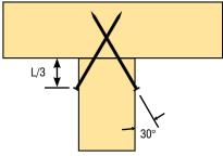
FIGURE B8-8 End jack to hip Girder Truss
