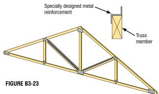
Permanent Building Stability Bracing for wind, seismic and/ or other lateral Loads acting perpendicular to the plane of the Trusses will always be needed in every Building.
