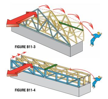
✓ Refer to BCSI-B1C, BCSI-B2C and BCSI-B7C for recommendations on proper bracing of Trusses.
