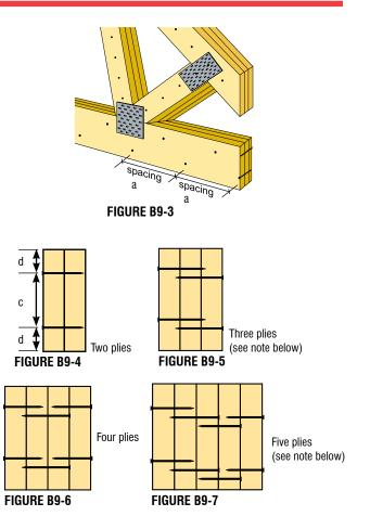
Girder Trusses of up to five (5) plies are permitted to be fastened together with nails. Nail each additional ply in accordance with the specified schedule found on the TDD. For four (4) and five (5) ply girder trusses all chord members must be bolted together using 1/2" diameter ASTM A307 Grade A bolts and washers per panel in addition to the specified nailing.
