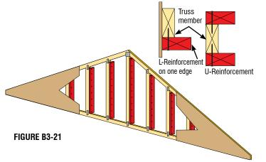
Scab Reinforcement is installed on one face of the Web. It is often more structurally efficient for multiple-ply Webs and provides easier nailing because it is applied to a wide-face of the Web.
