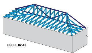
Alternate Option to Step 1 & 2: Assemble the Girder Truss and jacks on the ground and lift the entire assembly into place. Be sure to get guidance from a Registered Design Professional to ensure modules are designed and installed safely and properly (see page 28 for information on an alternative installation method).
